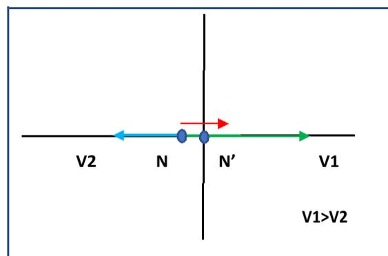
Fig. 3 Phasor diagram of split phase or single phase three wire system with unbalanced load.
