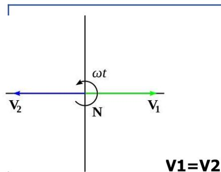
Fig. 2 Phasor diagram of split phase or single phase three wire system with balanced load.
