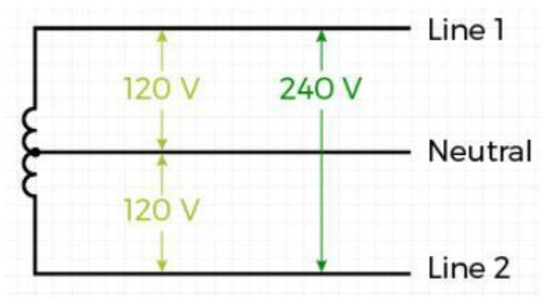
Single phase three wire system with hot lines and a neutral. Heavy-duty single-phase loads in commercial premises run from 240V L-L system (2 #Hot wires) and lower power equipment runs from 120V L-N system.
