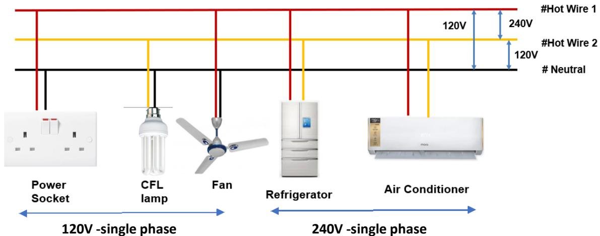
**Fig. 1 Uneven distribution of low power (@120V) loads in a commercial building**
